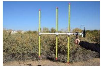
On the left, is a picture of the inexpensive directional antenna that I just described. I built one in about an hours worth of time. I don't remember the total cost but I would say it can be done for around \$10.
