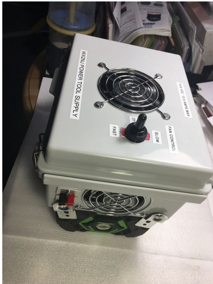
Bottom Right side of box showing Powerpole outlet and swing locks for battery of box with battery removed
