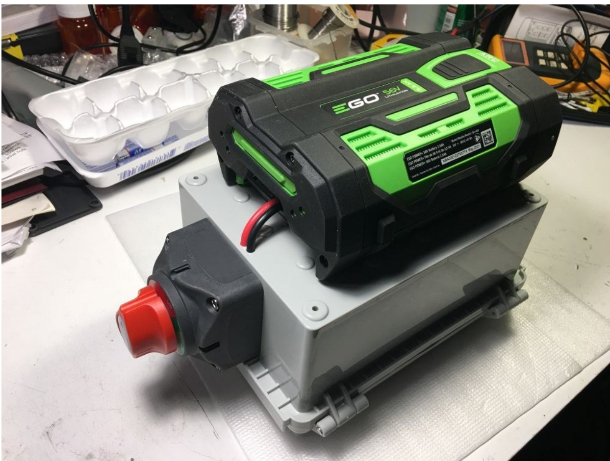
Bottom of box with EGO 2.5 amp-hour, 56 volt battery attached
