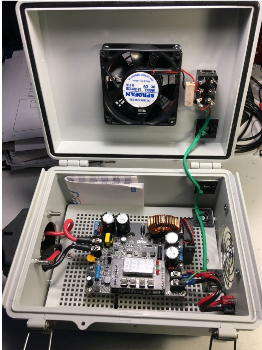
Interior view. Cooling fan blows air down into box.
